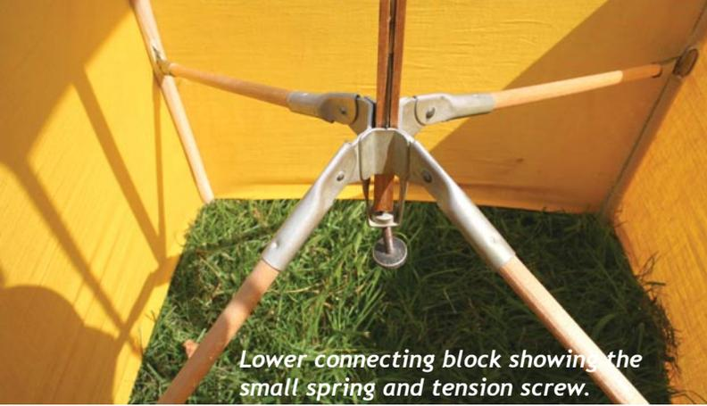
Lower connecting block showing the small spring and tension screw.
