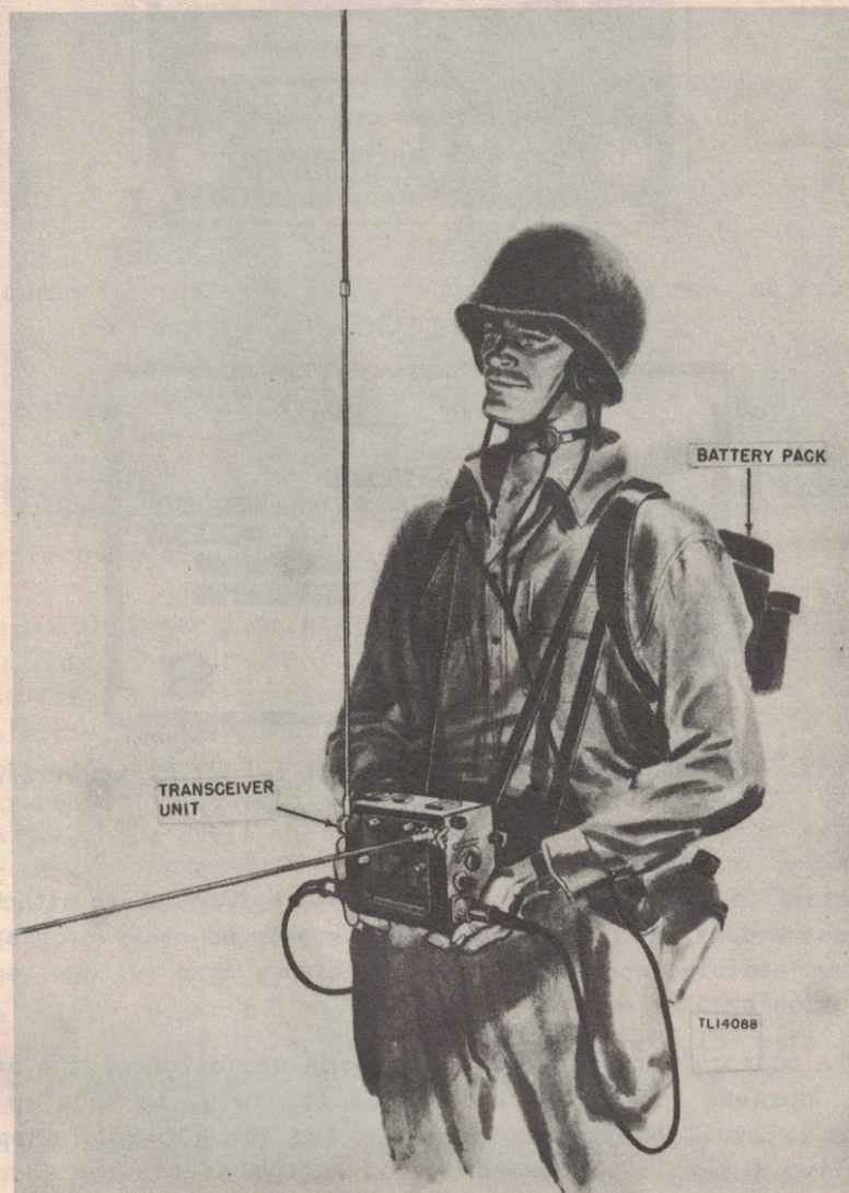
Figure 5. Japanese Radio Set Model 97 Light Wireless Set, portable operation by one man.
